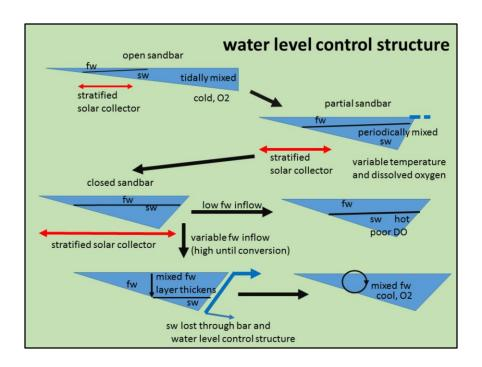
With a water level control structure that controls the lagoon height and also preferentially siphons and discharges bottom salt water from the lagoon, flooding can be averted and the lagoon can be converted to a mixed, productive rearing habitat for steelhead (and tidewater goby). Initial inflow should be relatively high to speed the conversion, but can be reduced after conversion of the lagoon to freshwater.
